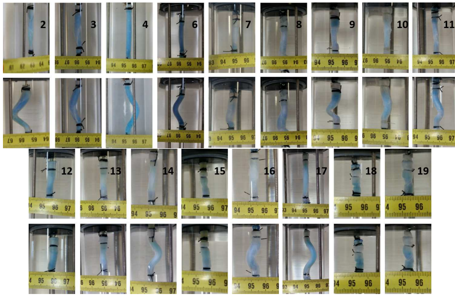
Figure 4: Photographs of all specimens included in statistical analysis (photo of specimen 5 is missing). In the first row of every group, the internal pressure is 0\text{mmHg} . In the second row of each group the internal pressure is \approx 240\text{mmHg} . Axial stretch ratio is 1 in all experiments, therefore inflation resulted in a "buckling-like" shape.
