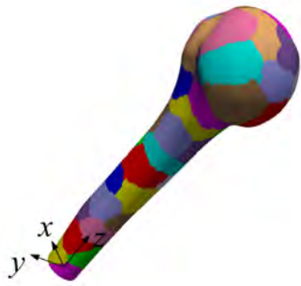
(a) Partitions of the mesh to 48 processors. (b) Slice of the bone with 48 partitions.
