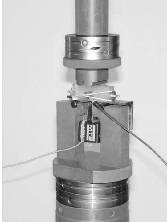
Figure 5. Four-point-bending test fixture with acoustic emission transducer and crack opening displacement gage (PMMA specimen).
